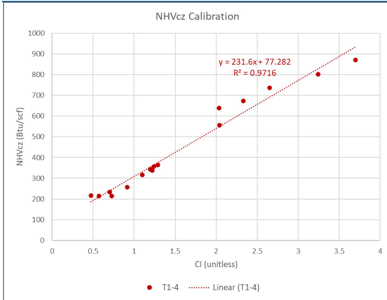
**Figure 3:** Instrument calibration using Tests 1-4.
