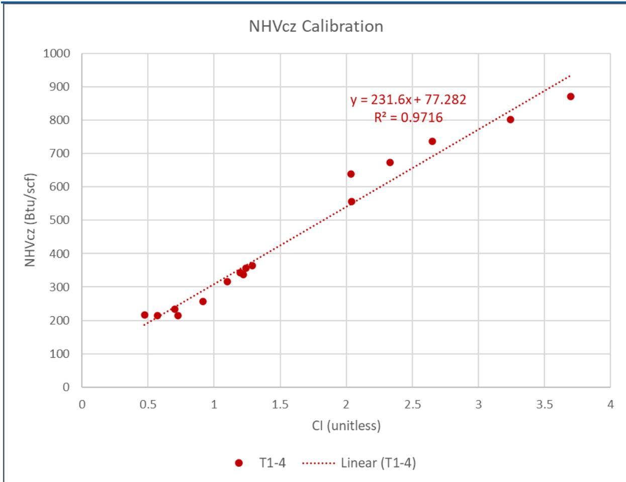
**Figure 3:** Instrument calibration using Tests 1-4.
