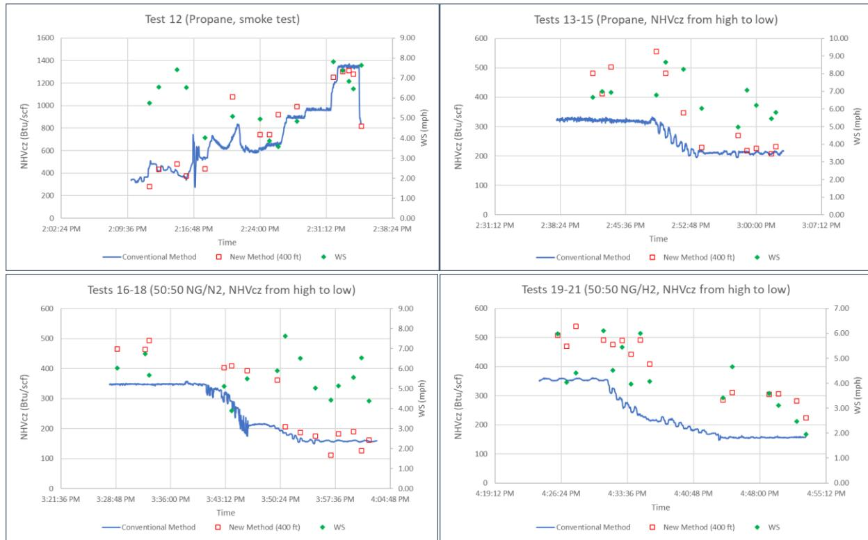
**Figure 6:** Flare NHVcz measured by the conventional method and the new method. Tests 12-21.
