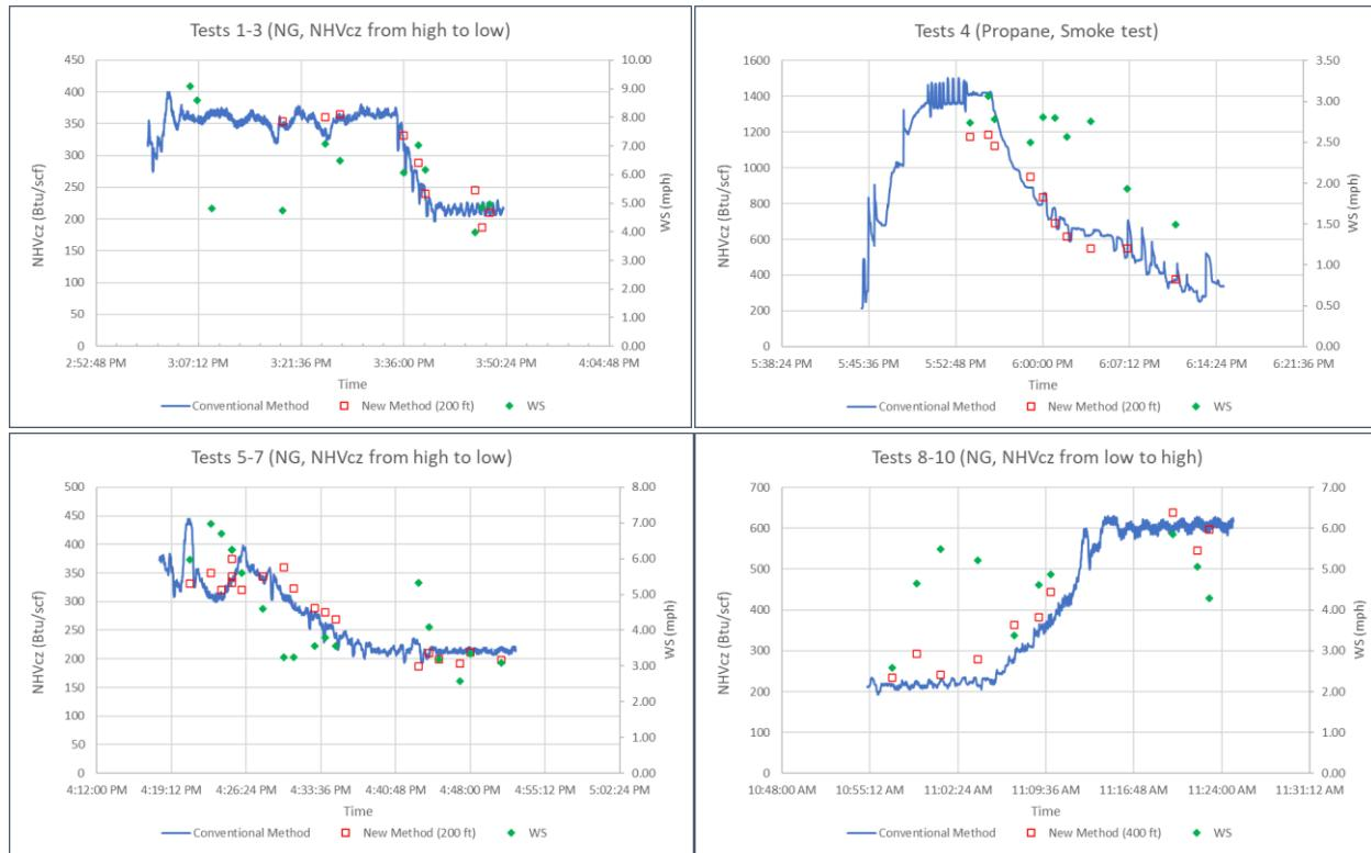
**Figure 4:** Flare NHVcz measured by the conventional method and the new method. Tests 1-10.
