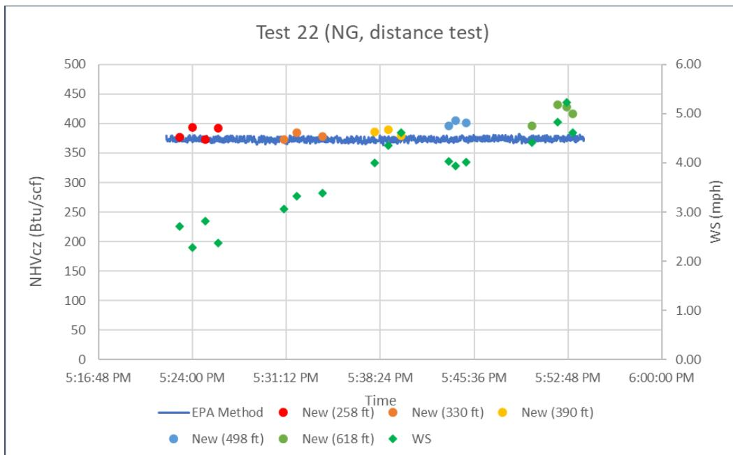
**Figure 7:** Flare NHVcz measured by the conventional method and the new method. Test 22.
