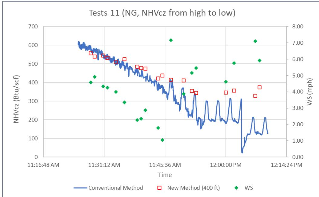
**Figure 5:** Flare NHVcz measured by the conventional method and the new method. Test 11.
