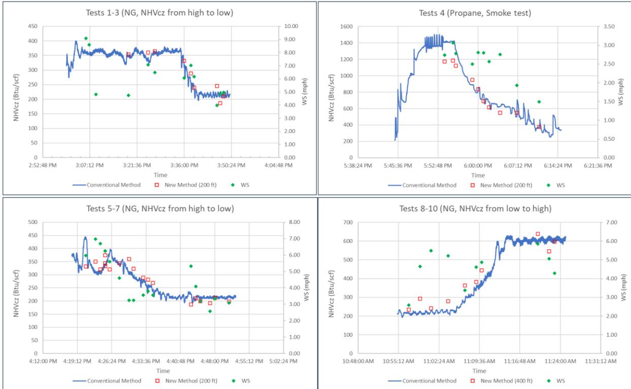
Figure 4: Flare NHVcz measured by the conventional method and the new method. Tests 1-10.
