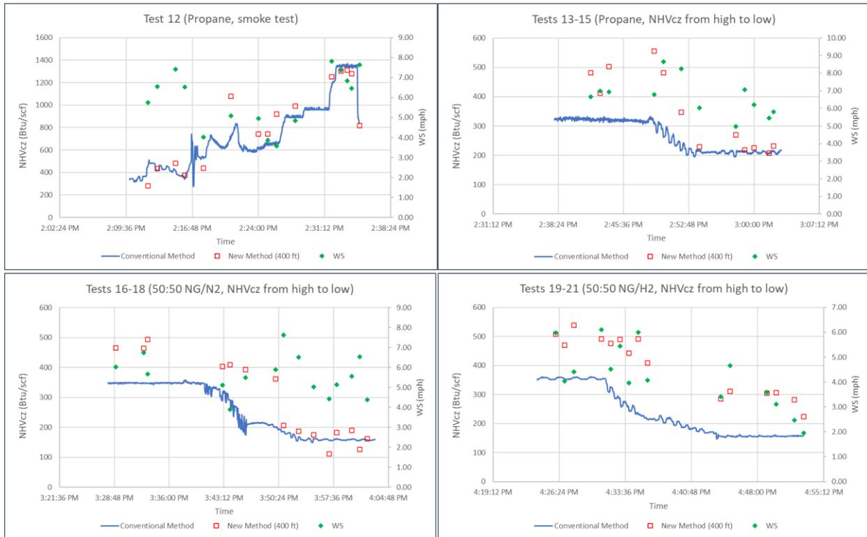
**Figure 6:** Flare NHVcz measured by the conventional method and the new method. Tests 12-21.
